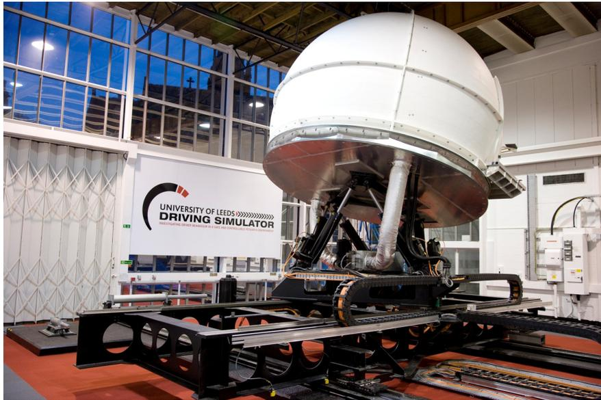
**Figure 62: The Leeds Driving Simulator**
