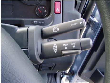
**Figure 27: MAN TGL cruise control column stalk**
