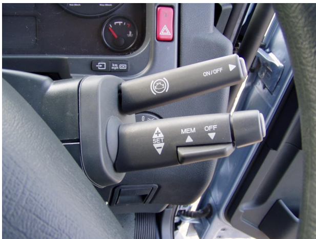
Figure 3: MAN TGL cruise control column stalk
