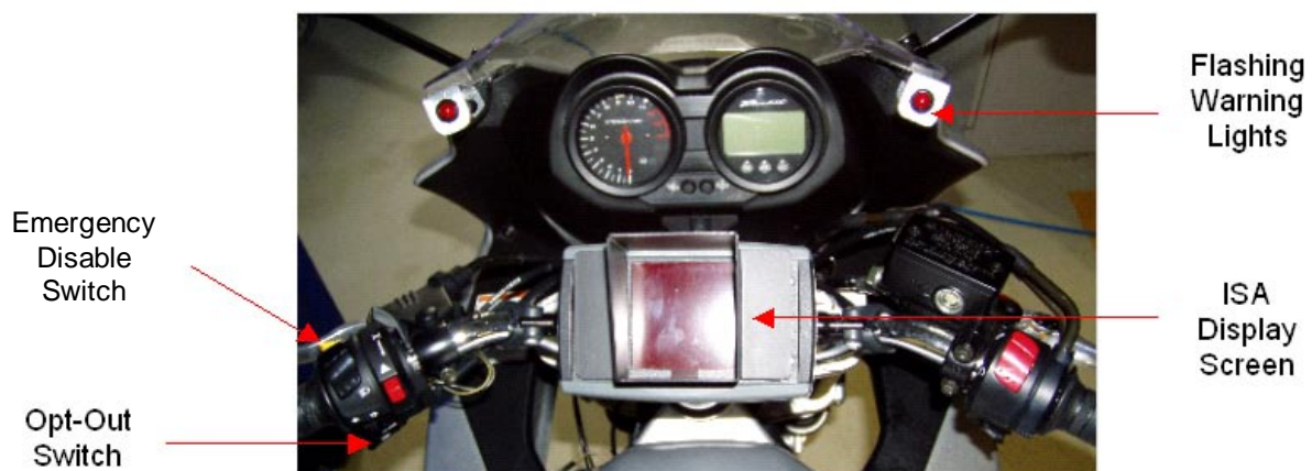
Figure 7: The ISA motorcycle system elements
