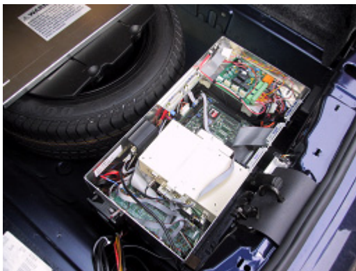
Figure 6: The main ISA equipment installed under the luggage storage area
