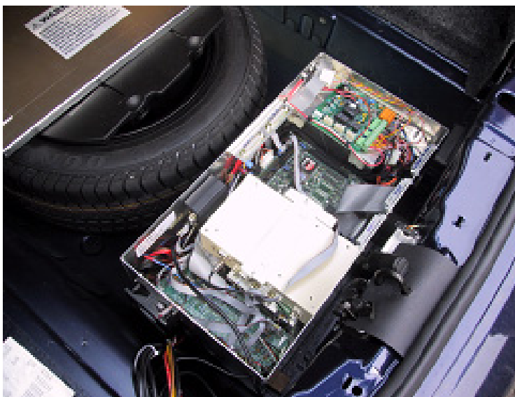
Figure 2: The main ISA equipment installed under the luggage storage area
