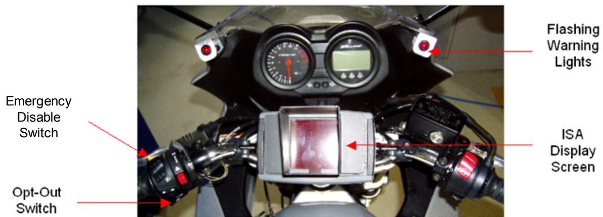
Figure 19: The ISA motorcycle system elements
