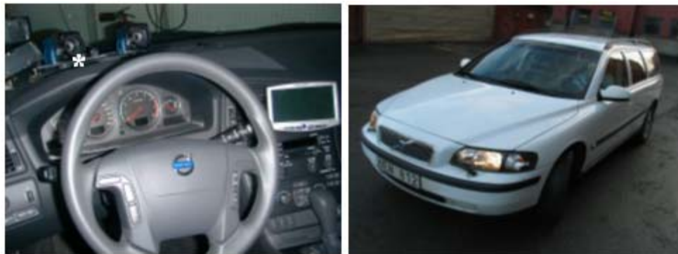
Figure 125 – Interior of vehicle with FaceLAB cameras on top of the dashboard (*) and exterior of the instrumented vehicle
