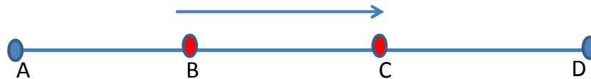
Figure 7: The test network. Trains enter at A and exit at D, while stopping en-route at stations B and C.
